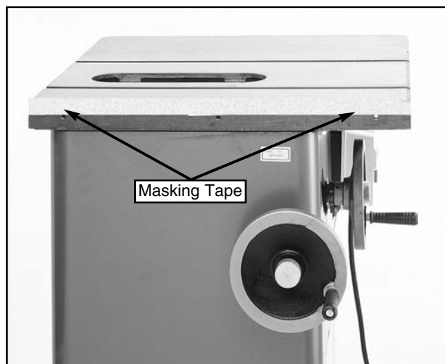
Figure 7. Using tape to shim for wing alignment.
